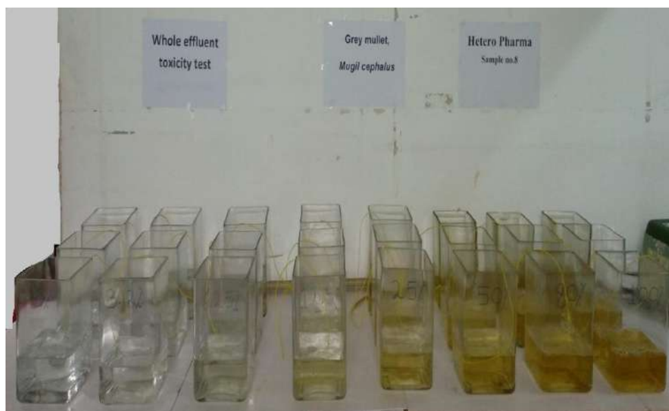
Fig. 4.4: Experimental setup used for 96 hr LC 50 of Hetero Pharma effluent with fingerlings of mullet ( Mugil cephalus )
